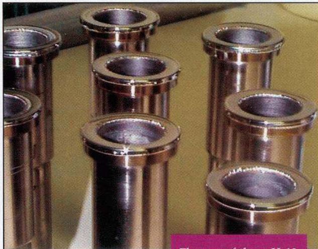
Flanges of these H-13 sleeves have been plated with .020 inch of NiColoy nickel-cobalt alloy. The addition of cobalt significantly strengthens the coating, according to the alloy's inventor, Berl Stein.
