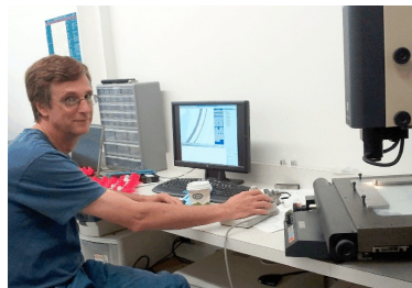
Precision electroforms are being inspected with the Smart Scope
