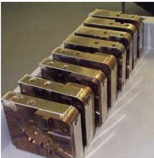
Figure 2 Mold Blocks Selectively Plated on two Sides with 0.040" of NiColoy™
