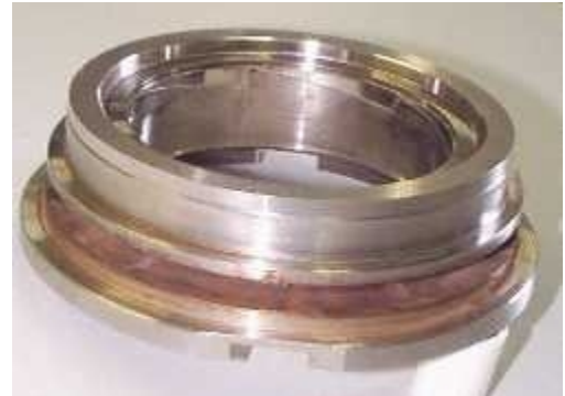
Figure 3 Sawtooth Areas Selectively Plated with .0005" of NiColoy™
