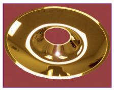
Eye spy. Pictured above is the first of several prototype primary mirrors AOS fabricated. Its unusual aspheric shape allows for a very wide field-of-view while still maintaining a central area of high resolution.
